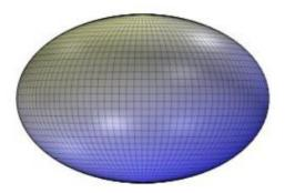
Ellipsoid/Sphere  $\frac{x^{2}}{a^{2}} + \frac{y^{2}}{b^{2}} + \frac{z^{2}}{c^{2}} = 1$ (ex: 3x<sup>2</sup> + 5y<sup>2</sup> + z<sup>2</sup> = 3)
